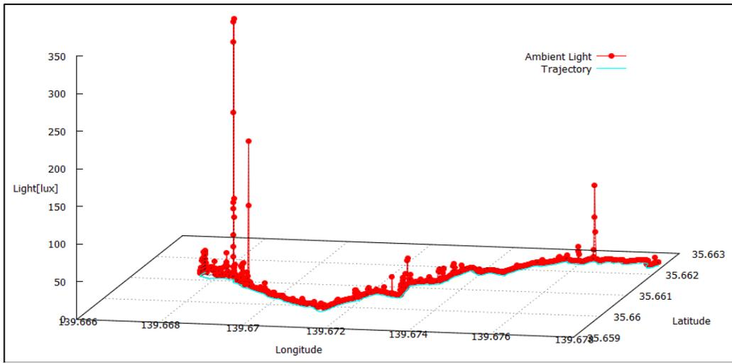
Figure 4: Ambient light along trajectory (Samsung nexus s)
