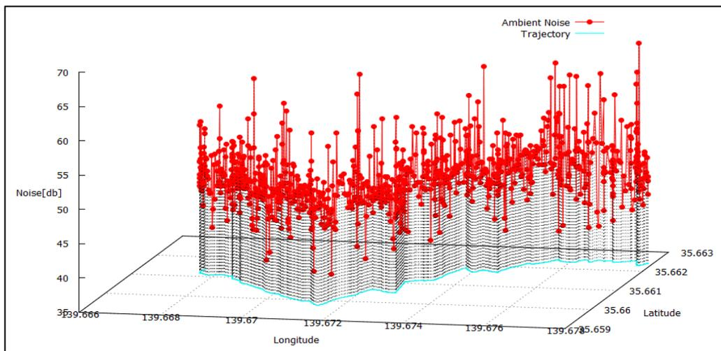
Figure 6: Ambient noise along trajectory (Samsung nexus s)
